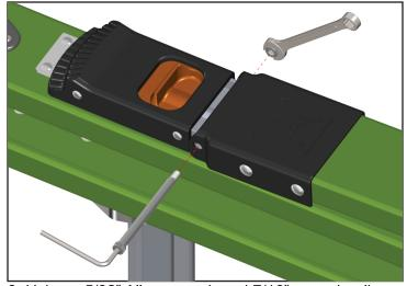
3. Using a 5/32" Allen wrench and 7/16" wrench, align and tighten the new shoulder bolt and lock nut.
