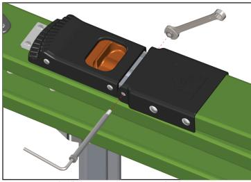
2. Using a 5/32" Allen wrench and 7/16" wrench, remove and discard the existing shoulder bolt and lock nut
