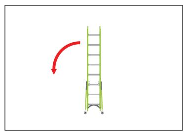
1. Lay the ladder on its side with the bolt being replaced facing up.
